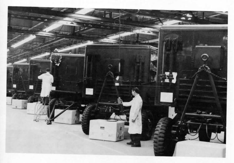
Fault isolation trailers, seen here in final assembly, are used for countdown checkout and centralizing of fault or error within the ground support unit.
