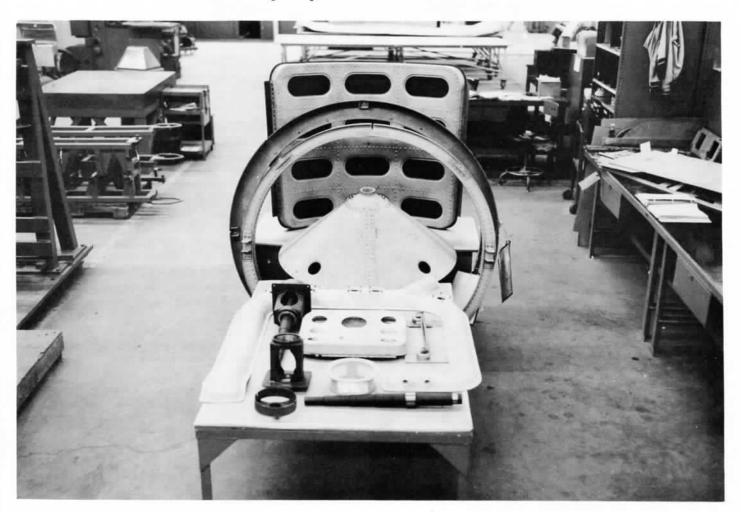
Some ready-to-assemble component parts are grouped here. They include the instrument panel door, payload support rings, door, and cone support. Dark parts are the vane drive assembly (neg. 31571).
