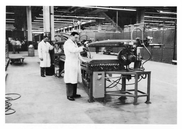
For the tail section a corrugated skin is used. It is cut to length and width in the manner shown here (neg. 31511).
