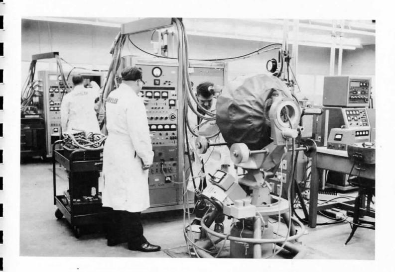
Specialists calibrate a gyro-stabilized platform on a planetary test stand in one area of Guidance and Control Laboratories. Here, hand-picked engineer-technician teams develop systems for delivering the "punch" on target (neg. 31579).
