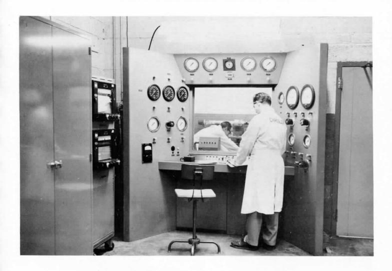
In this high-pressure test room — one of the many facilities of the Mechanical Laboratories — pneumatic systems of all missile components are checked out (neg. 31578).
