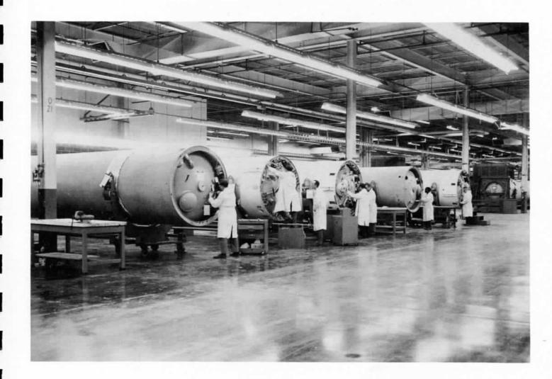
After the center section has been built up much the same as the aft part, electrical specialists install the harness assemblies (neg. 31541).
