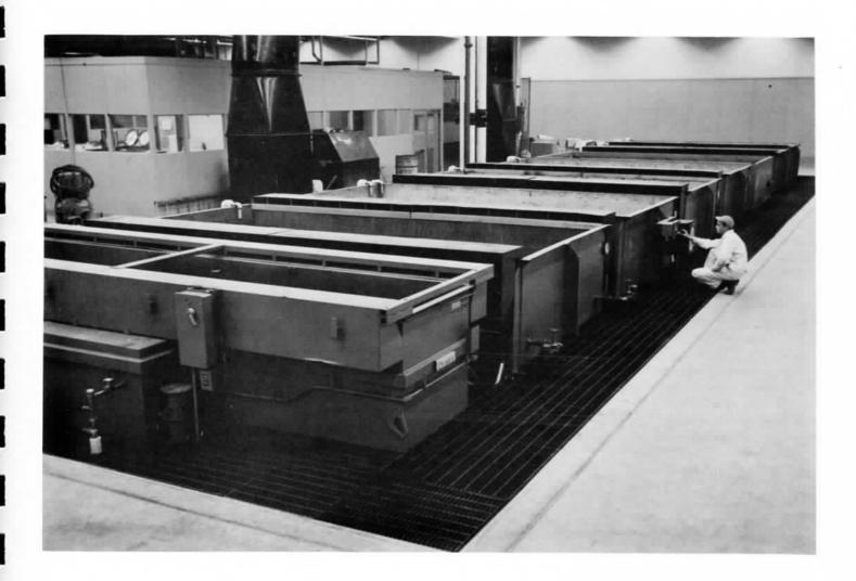
In addition to plating tanks, the plant has recently installed complete tank equipment for degreasing, as well as aluminum anodizing tanks (neg. 31570).
