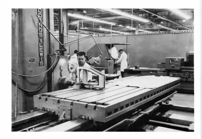
One of the outstanding machines is the large Giddings and Lewis milling machine, shown here working a valve box (neg. 31495).
