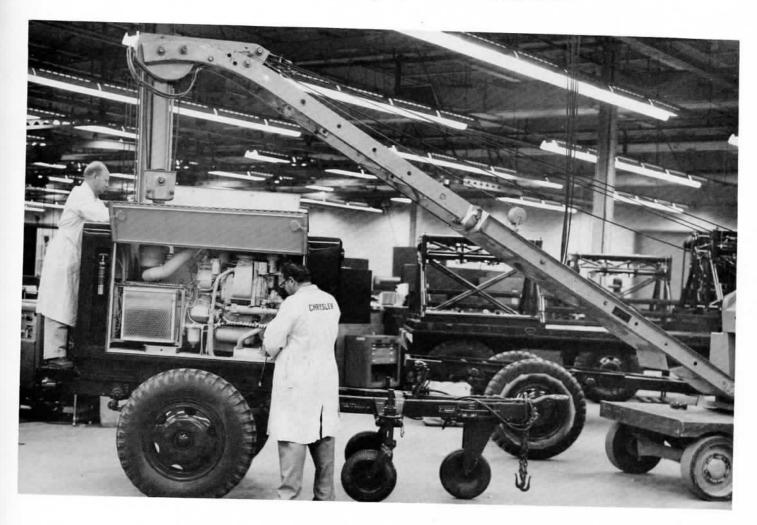
This 30-watt generator, which is assembled at Chrysler Missile Division, supplies all the power tor lighting, at the launching site.
