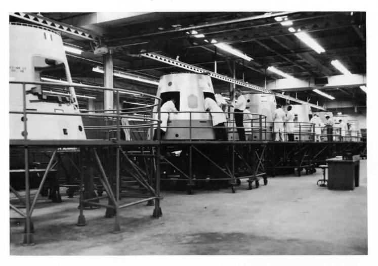
With metal work completed on the aft section, instrumentation, installation, and finish buildup are handled assembly-line fashion, on a row of stands (neg. 31506).
