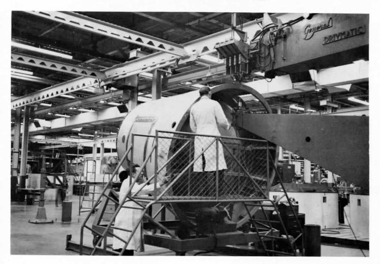
Here a metal circle or skirt has been welded on the base of the upper piece. This large special machine automatically drills and rivets support rings inside diameter of the cone (neg. 31513).
