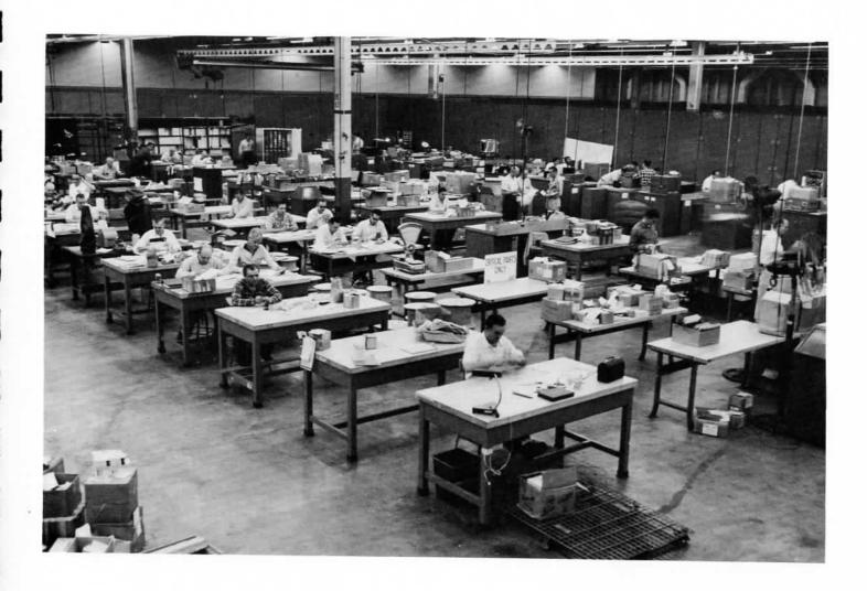
Important to the success of missile production is this group of inspectors in the large Receiving area. Here, incoming component parts are checked with precision instruments before acceptance (neg. 31527).
