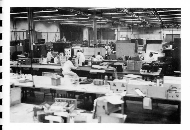
This area, fully equipped with test instruments, checks out the electrical assemblies before they are installed as missile components (neg. 31550).
