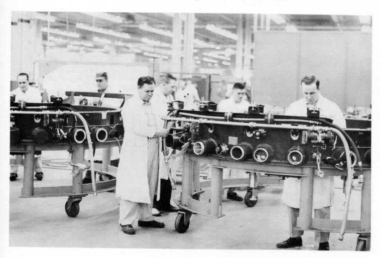
This is the final assembly area for auxiliary launching rings.
